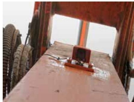
Top: Camera in the jib for work space monitoring. Centre: Camera for side monitoring. Bottom: Camera for rear space monitoring.
