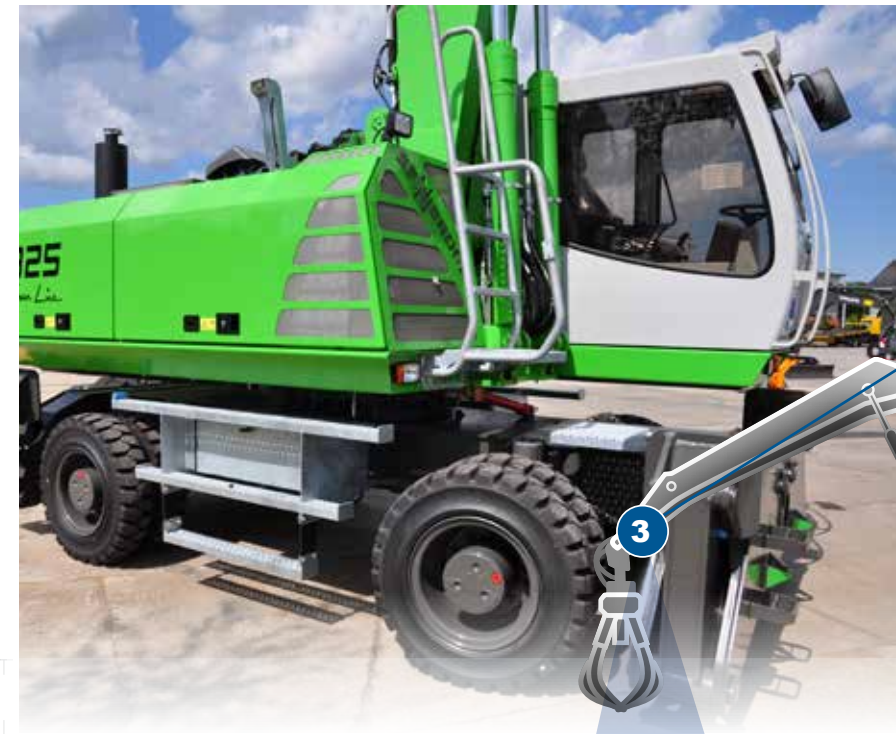
Mobile material handling digger, fitted with a complete Motec camera and monitor system.
