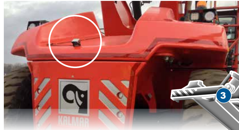
Bottom: Motec rear camera – very important for the highly agile reach stackers.
