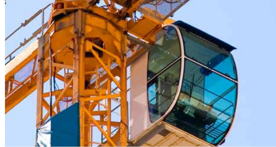
Detail view of a top-slewing tower crane with cabin. The motor zoom camera and the radio transmitter are mounted at the crane carriage.
