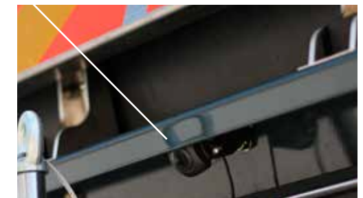
Putzmeister concrete pump truck with front camera, ultrasound and radar sensor, side monitoring and rear space monitoring.
